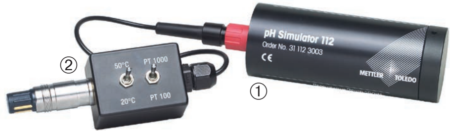
pH Analog Verification Kits: Combining the pH simulator 112 ① with the VP simulator ② both pH and Temperature signals can be simulated to check the automatic temperature compensation capability of the transmitter.
