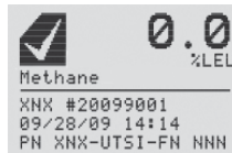
Figure 40. General Status screen with unit information
