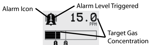
Figure 34. General Status Alarm - detail
