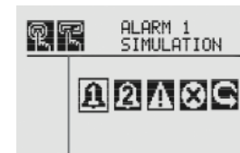
Figure 16. Alarm/Fault Simulation Menu
