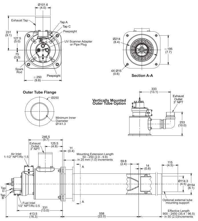
Version 5 outer tubes have a larger diameter flange than previous versions. Contact factory for retrofit of the burner to previous version outer tubes.
