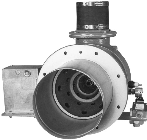
Fig. 4. View into metallic cone of Model EB-3 OVENPAK®-II Burner, arranged for external blower source, with connecting base and linkage assembly to adapt customer's automatic control motor, and optional low fire start switch arrangement. Inlet air piping uses flexible connector set.
