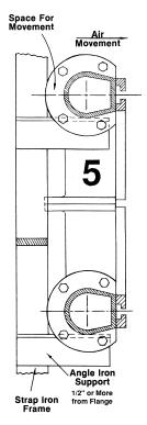
**Sketch 4** shows the burner suspended from a strap iron frame using USB (universal support brackets) supplied by Maxon. Note that rigid mounting is avoided by the 3/4" bracket hole which slips loosely over a 1/2" bolt or steel rod attached to the support. Gas piping would need independent support.
