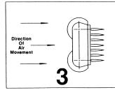
Maintain smooth, even air flow over the burner by designing supports to provide minimum interference, deflection and turbulence. Flat strap iron (with its width parallel to the direction of movement) is preferable to angle iron or channel supports.
