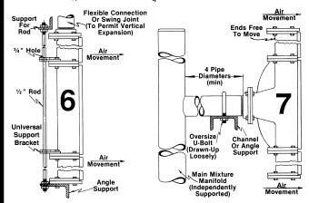
**Sketch 6** shows angle iron used to support the burner. Note that narrow edge of angle faces air flow.
