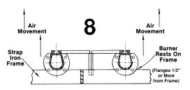
Support for down-fired burners can be accomplished as shown in the illustration at right. Always avoid rigid mounting.
