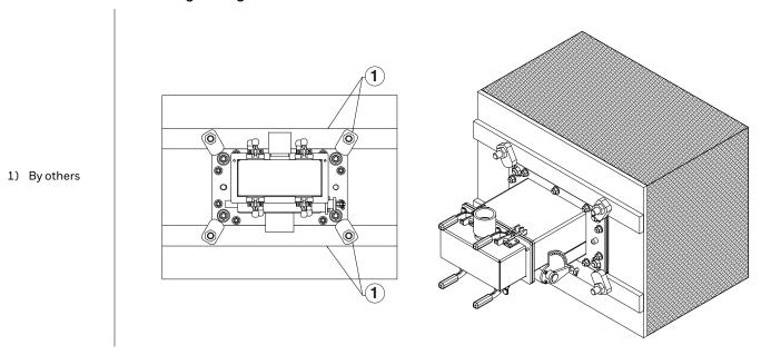
Burners should not be installed in a down-fired position.
