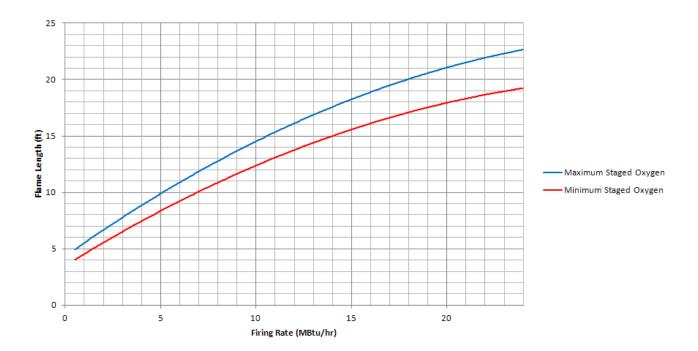
Flame lengths shown are typical for burners sized and operating at maximum design conditions. Flame lengths per unit of heat input will vary from these values when burners are operated below maximum design.
