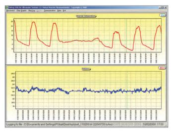
THIS CHART SHOWS HOW A MEASUREMENT OF DISTANCE VARIES (LOWER TRACE) AGAINST CHANGES IN TEMPERATURE OVER THE PERIOD OF A WEEK. DESPITE TEMPERATURES RANGING FROM OVER 25°C DOWN TO -7°C, THE MEASUREMENT REMAINED EXTREMELY CONSTANT, WITHIN  $\pm 0.5$ MM, ON A RANGE OF 383.5MM.
