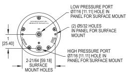
Combining clean design, small size and low cost with enough accuracy for all but the most demanding applications our SERIES 2-5000 Minihelic® II gage offers the latest in design features for a dial type differential pressure gage. It is our most compact gage but is easy to read and can safely operate at total pressures up to 30 psig.
