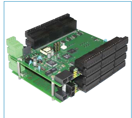
ESA-OMK open board stacking kit. One kit supplies standoffs to stack two units.
