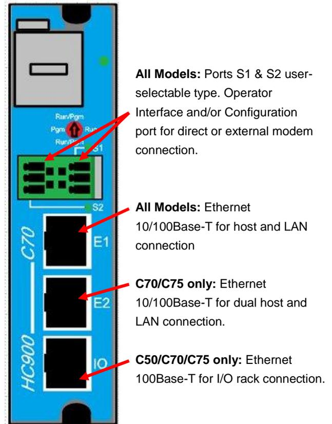
**Figure 1 Communication ports**
