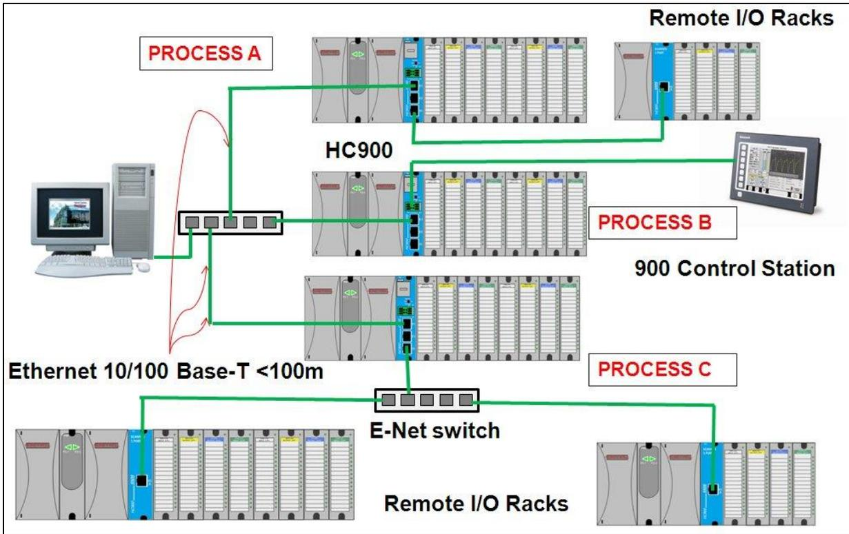
Figure 4 - MULTIPLE PROCESS/MULTIPLE RACKS – PROCESS
