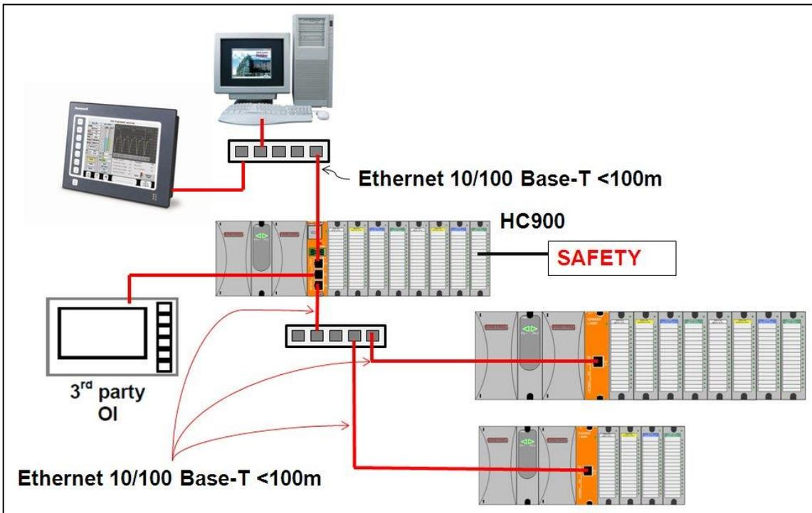
Figure 3 - SINGLE PROCESS/MULTIPLE REMOTE RACKS- SAFETY
