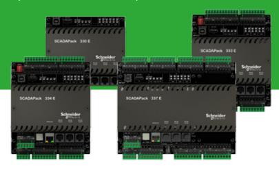
The SCADAPack™ 300E Smart RTU is a platform built on a 32-bit processor and fitted with a 12...30 Vdc supply, various communication links and a wide range of analog and digital I/O that adheres to open standards and can operate in the harsh demands of a remote environment.
