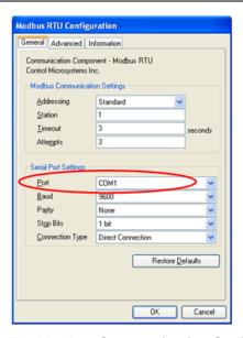
The **Modbus Communication Settings** grouping contains Modbus specific communication settings.
