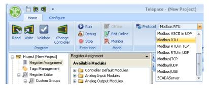
Check that **Modbus RTU** is selected and click the **Settings** button. The **Modbus RTU Configuration** dialog is opened.
